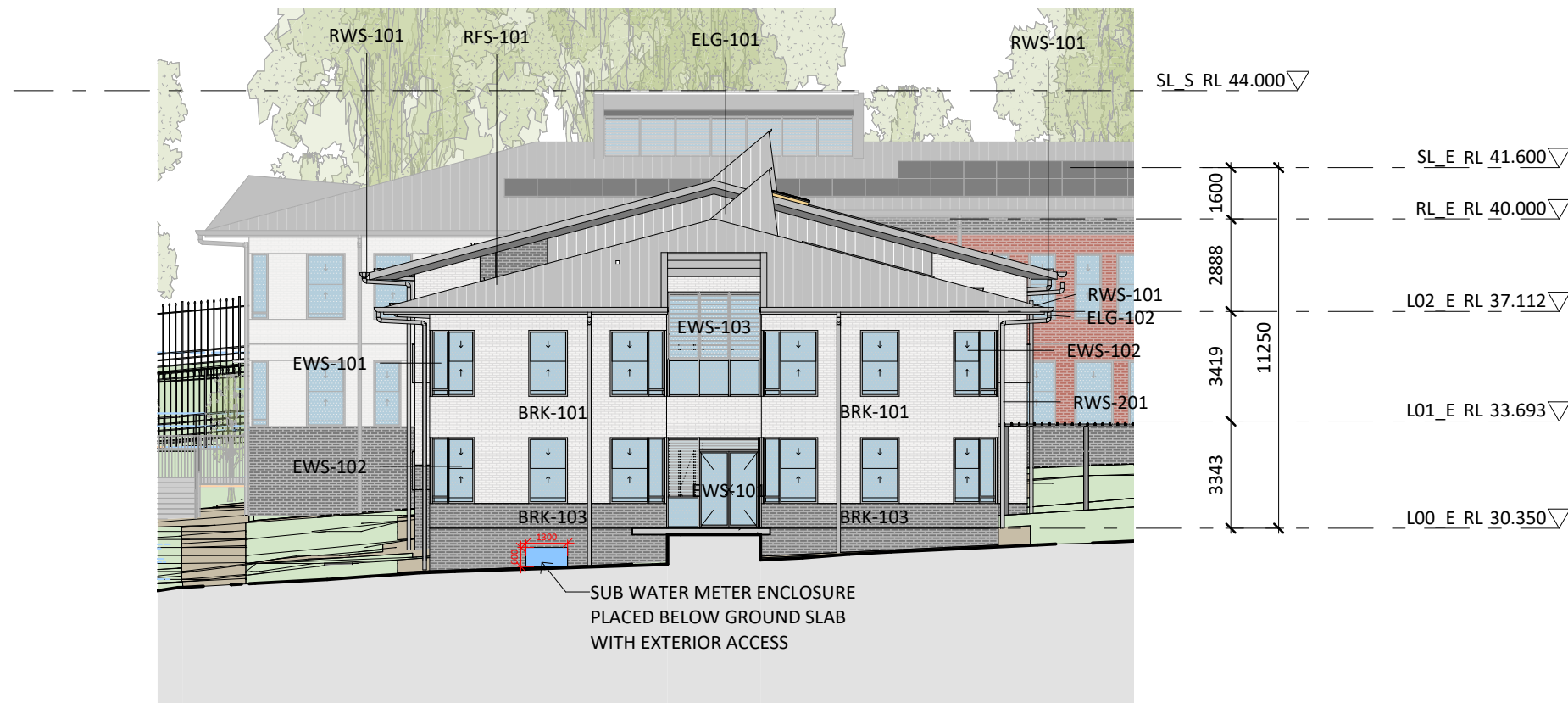
3 ELEVATION - BLOCK U - EAST 1 : 200 @A1
