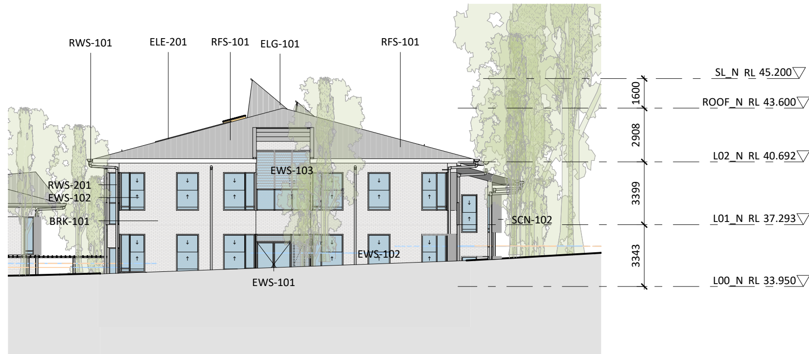
1 ELEVATION - BLOCK T - NORTH 1 : 200 @A1
