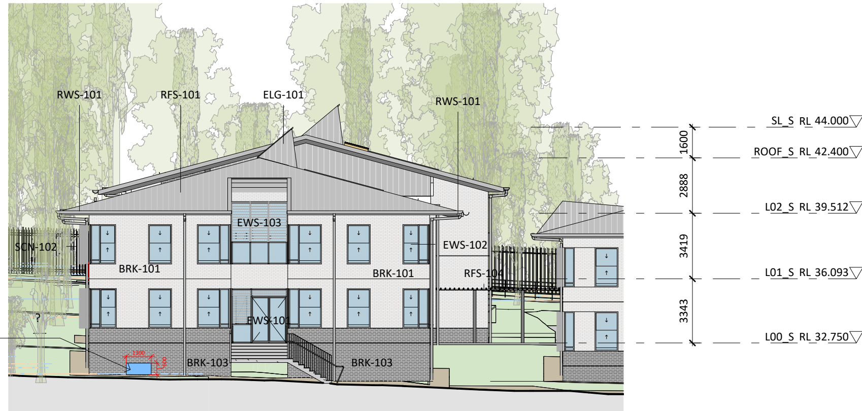
2 ELEVATION - BLOCK T- SOUTH 1 : 200 @A1
